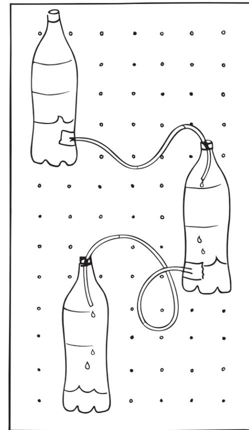
Test your design by pouring water into the first bottle; pressure will build up and push the water through the tubing into the next bottle. It may not work the first time, so just adjust the placement of your bottles and tubes until the water starts flowing!
