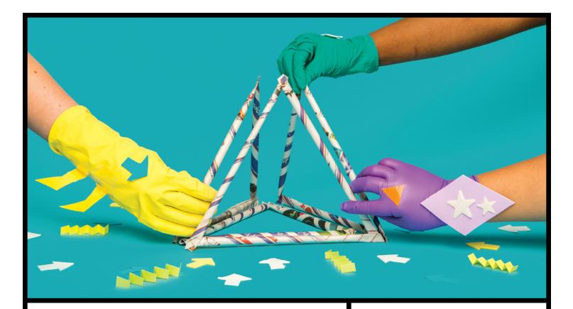
Triangles are considered the strongest shape because they can handle heavy loads without collapsing. Hold one of your newspaper triangles and apply some force on the sides; the triangle should feel sturdy and hold its shape. If you put force on a square or rectangle, the shape can tilt or collapse. The triangle's strength is why architects use it often in structures.
