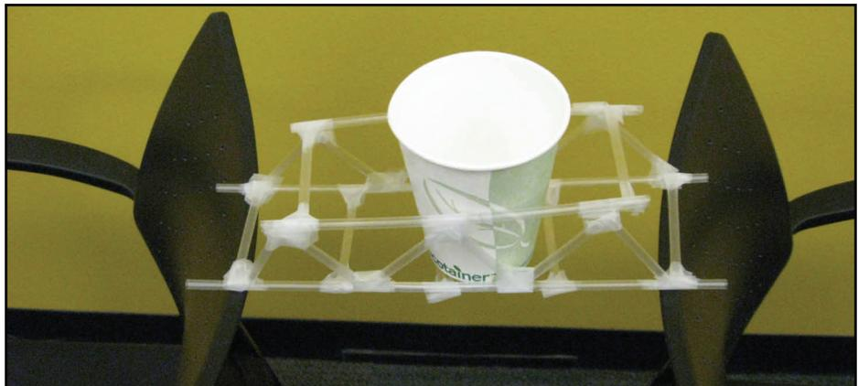
8. Gradually fill the cup with pennies until the bridge either collapses or bends down 9 cm (where the “water” would be).
