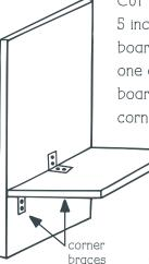
Cut the wood into three pieces – two that are 5 inches long and one that's 14 inches. The 14-inch board is the backboard. Measure 3 inches from one end of the backboard and connect a 5-inch board perpendicular at that point, using the corner braces. Use two corner braces on the
