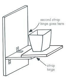
Test the tipping shelf by holding the backboard vertical (such as against a wall) and filling the container with water. The container should tip with a gentle nudge. If it takes too much force to tip, reposition the container away from the backboard so that its center is right over the hinge. If the container won't stay put and always tips, reposition the container towards the backboard. The key is to have the center of mass just behind the hinge pivot.
